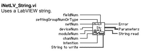
String to write String The value to write to the specified field within the instruNet World.
