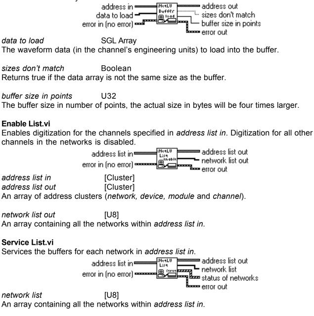
*status of networks* [Cluster] An array of the *network status* cluster (see **Service All Buffers 2.vi**). The data for each element of the array is from the network specified in the corresponding element of the *network list* array.
