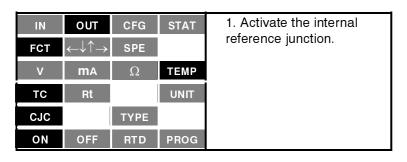
The function simulates a compensated thermocouple according to the room temperature.
