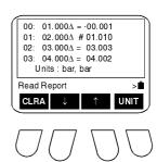
Symbol # appears when the result is incorrect, i.e.: when the computed deviation is higher than the authorized deviation. In this example, the transmitter will be considered as discrepant. By default, setpoints and deviations are displayed in physical unit emitted by the CL519. Nevertheless, the deviation can be displayed in electrical unit measured by the CL519.
