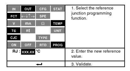
The function simulates a non-compensated thermocouple with a reference junction different from  $0^{\circ}\text{C}$ .
