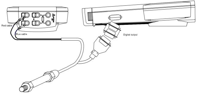
Each setpoint emitted is displayed in the OUT window. In reality, there is no setpoint emitted on the OUT terminals of the CL519, the unit only displays (and if required stores) the setpoint value emitted by the pressure generator and measured by the module CL519-ACL333.
