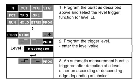
Overrun of a level always triggers an automatic measurement burst such as programmed.
