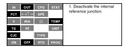
In this case, the function simulates a non-compensated thermocouple with a reference junction at  $0^{\circ}$ C.
