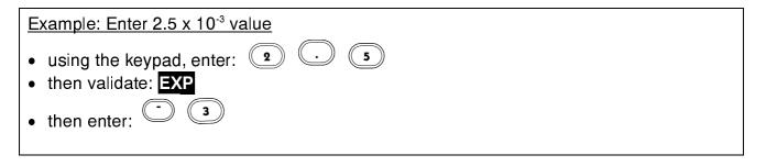
In case several variables are necessary, changing to the next (or previous) parameter is done by validating the >> ( << ) prompt using the function key.
