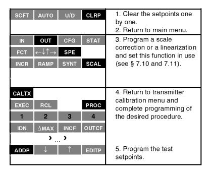
NOTE: When a setpoint is programmed, it is accepted only if it meets the emission range of the procedure. So do take care when changing the emission range (see § 8.6.1) after the setpoints are programmed because setpoints could not be compatible with the new range.
