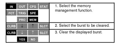
When a measurement burst is cleared, its order number is assigned to the next burst. Consequently, the order number of all next bursts is decremented of one unit.
