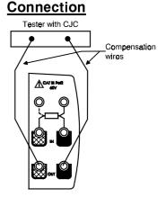
WARNING: After an important heat shock, we suggest you allow the unit to settle in temperature before using the internal reference junction (CJC) in order to get the max. accuracy.
