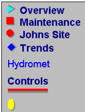
Global alarm button shapes, and colors. Text can also be a global alarm button.
