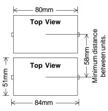
The Proper Installation & Maintenance of TX801DC.
