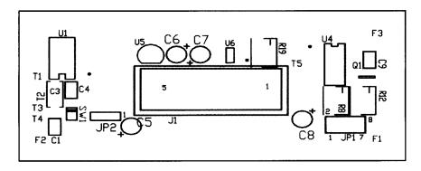
R19- OFFSET ADJUSTMENT R12- GAIN ADJUSTMENT R8 - SCALE ADJUSTMENT
