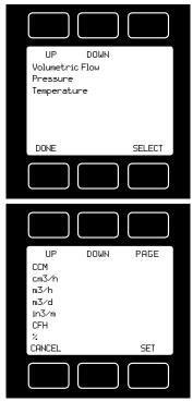
Press **DEVICE UNITS** to access menus of units of measure for each parameter (and totalizer if so equipped).
