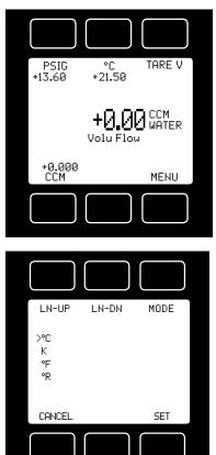
This mode defaults on power up, with flow as the primary displayed parameter. The following parameters are displayed in the Main mode.
