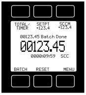
TIMER button will cycle the large numbers on the display between total mass and time elapsed.
