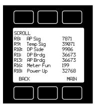
**DIAG TEST:** This diagnostic screen displays the current internal register values, which is useful for noting factory settings prior to making any changes. It is also helpful for troubleshooting with Omega customer service personnel.
