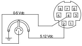
50 KOhm Potentiometer Controllers: A simple method for providing set-point to controllers
