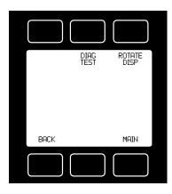
MISC2 will display as shown at left. Press ROTATE DISP and SET to Inverted 180° if your device is inverted. The display and buttons will rotate together.
