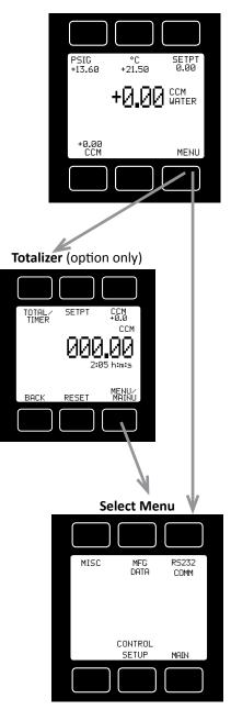
The **Main** display shows, temperature and volume flow. Line pressure will be also be displayed if the meter was order with this option.
