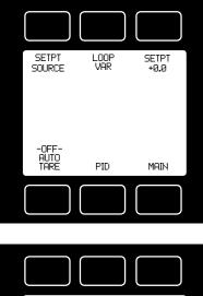
LOOP VAR—Water flow controllers are defaulted to volume flow. Volume means that the controller is "closing the loop" on the volume flow rate. This means that when you give the controller a set-point, the controller compares that set-point to the measured volume flow rate and adjusts the valve to try to make the flow and the set-point match. For the volume flow rate, the input signal (e.g. 0-5 Vdc) corresponds to the full-scale flow rate for the device.
