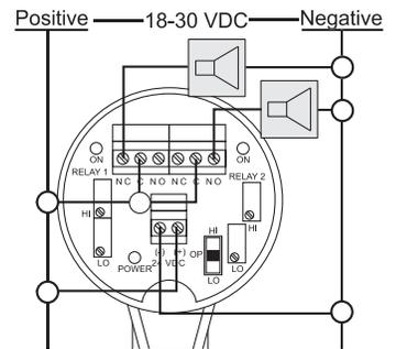
**Note:** Low level alarm is wired NC and the high level alarm is wired NO.
