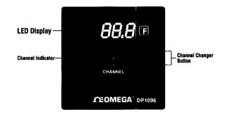
LED Display: This is the screen in which the temperature will be display.
