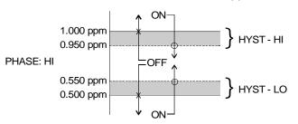
When value falls to  $\leq$  1.000 ppm, relay closes, until rises back to  $\geq$  1.050 ppm.
