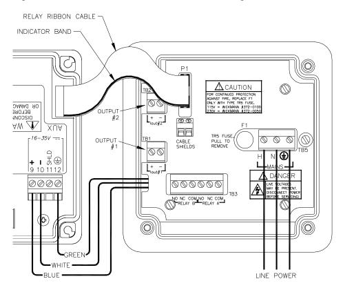
Figure 4-3 Line Power Connection
