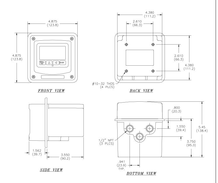
Figure 2-1 Enclosure Dimensions, AC Powered Units
