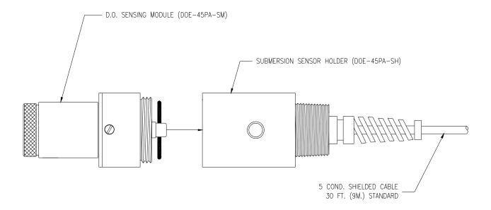
Figure 5-1 Submersible Oxygen Sensor Assembly
