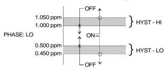
When value falls to  $\leq$  0.500 ppm, relay closes, until rises back to  $\geq$  0.550 ppm.
