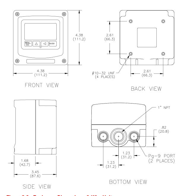
Figure 2-2 Enclosure Dimensions, 2-Wire Units
