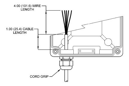
Figure 4-5 Sensor Cable Preparation
