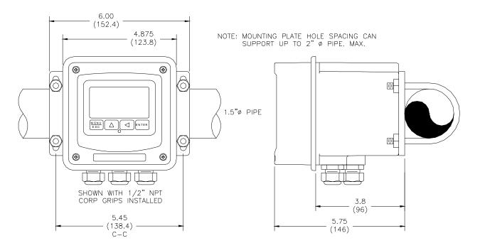
Figure 2-5 Pipe Mounting Diagram
