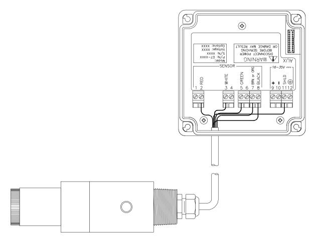
Figure 4-2 Submersible Sensor Connection
