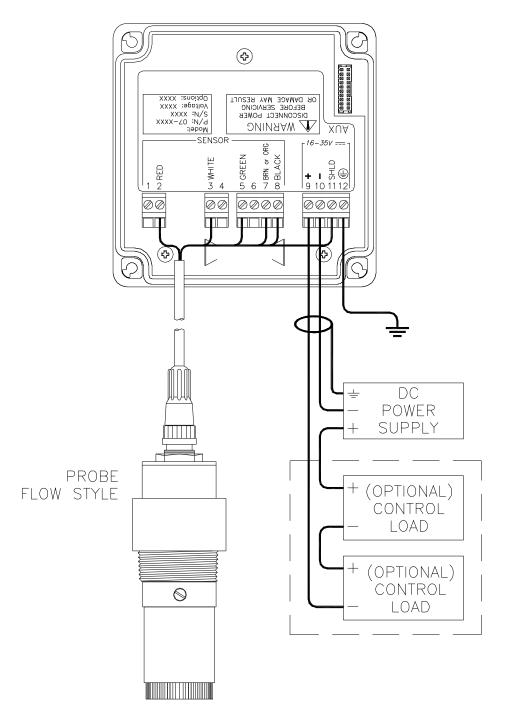
Figure 4-1 Loop-Power Connection
