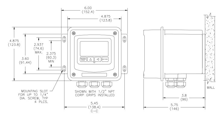
Figure 2-4 Wall Mounting Diagram
