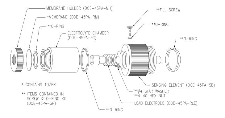
Figure 5-2 Submersible Sensing Module Assembly
