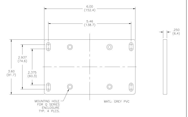
Figure 2-3 Wall or Pipe mount Bracket
