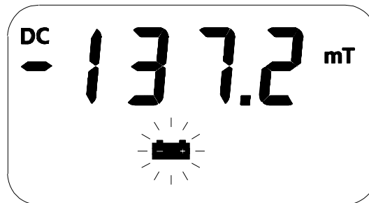
Figure 3-8 Low Battery Indication
