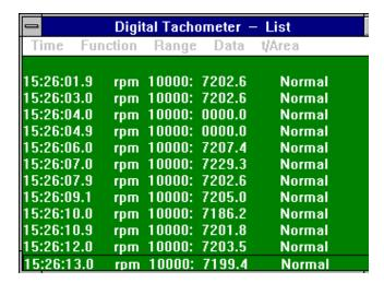
If this option is selected or CTRL+L is pressed, a window, which lists the date, function, range, and value every sampling, shall appear on the screen.
