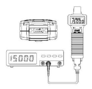
**NOTE:** It is strongly recommended that the emiting/receiving unit be covered to avoid undesired light signal coming in.
