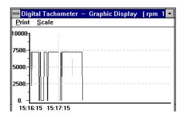
If this option is selected or CTRL+G is pressed, a window, which emulates strip chart recorder, shall appear on the screen. The graphic window has two menu, PRINT and SCALE. Select the PRINT menu, the graphics will be printed through any printer connected to the PC. The SCALE menu allows user to set
