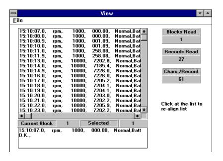
If the View option under FILE in the Main Window is selected, a view window will be shown as above, and the users can review your ASCII data file. If a printer is connected to the PC, users can print out content selectively.
