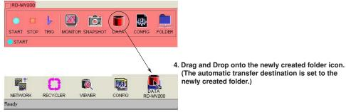
The data residing in the internal memory or external storage medium of the RD-MV can be automatically transferred to the specified folder on the PC.
