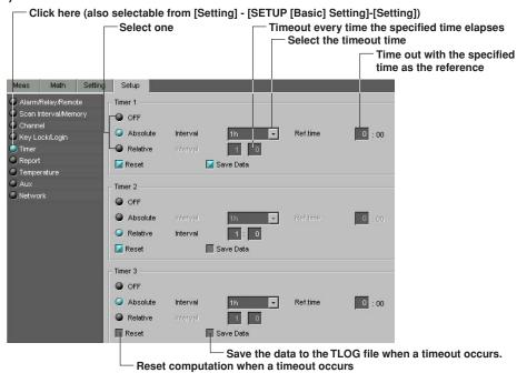
You can set three types of timers to be used in the statistical computation. You can have the data saved to a TLOG file or reset the computation when the specified timeout time elapses.
