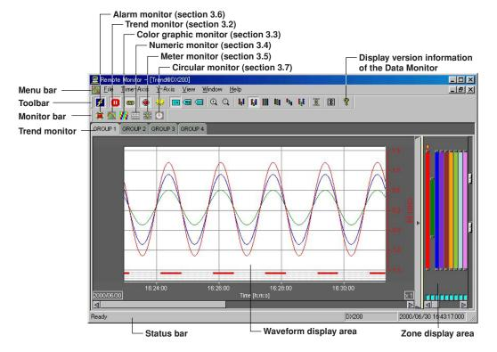
The Data Monitor can be used to monitor the measured/computed data and the alarms of the RD-MV100/RD-MV200. The following six monitoring methods are available:
