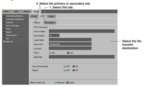
By using the FTP function, you can automatically transfer the measured/computed data files to the specified server.
