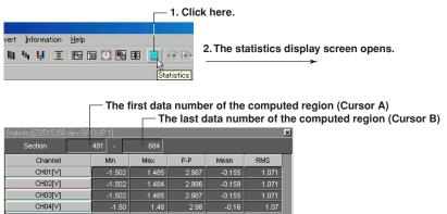
The minimum value, maximum value, P-P, mean, and rms value for each waveform in the range specified by Cursors A and B are computed and displayed. If the cursor is not displayed, the computation is performed over the entire data.
