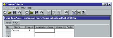
**6.** Enter the measurement interval with numeric characters and colons ":" (Example: 00:10:00).
