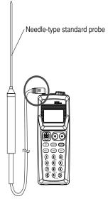
An example of the needle-type standard probe connected to input channel "A"
