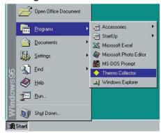
Select "Thermo-Collector" in the "Programs" accessed from the "Start" menu. After the main screen of the software is displayed, the "Setup Tags/Logs - New" screen will be displayed.
