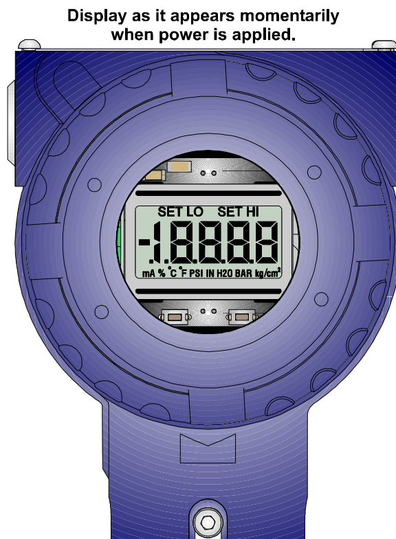
Figure 2-4 - Transmitter with Loop Powered Indicator Option Installed
