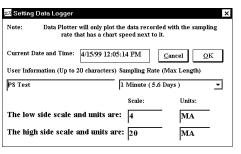
connected to a 4 ma to 20 ma transmitter and the transmitter will be converting the output of the transducer to a 4 ma to 20 ma signal.
