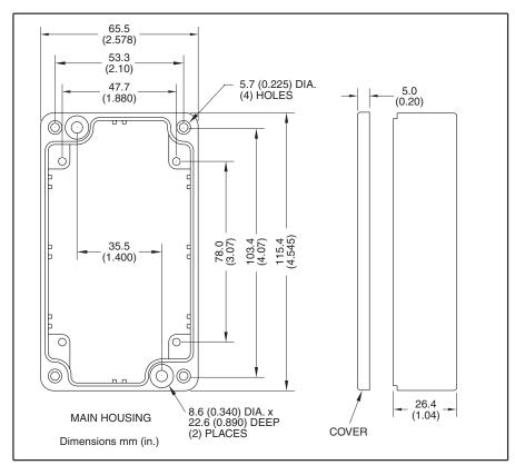
Figure 3-11. NEMA-4 Aluminum Enclosure
