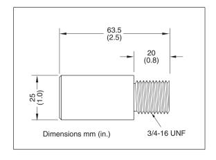
Figure 3-2. Sensor Housing
