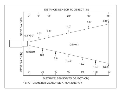
Figure 3-3. Optical Field Of View
