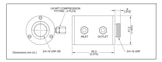
Figure 3-7. Water Cooling Jacket, OS100-WC
