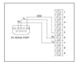
Figure 3-5. RS232 PC Interface Connection
