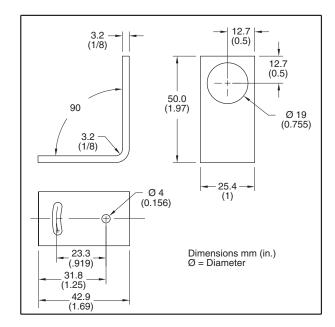
Figure 3-6. Mounting Bracket OS100-MB
