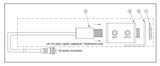
Figure 3-8. Typical Water Cool Jacket Assembly
