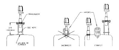
NOTE: MINIMUM 3" (76.20mm) ID FOR 3/4" (19.05mm) SENSOR MINIMUM 6" (152.40mm) ID FOR 2" (50.80mm) SENSOR
