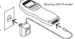
4 When the gauge is turned off, make sure the AC adapter/charger is disconnected.
