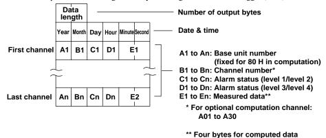
The data are output in the following format by receiving TS0 + "Device Trigger (GET)" + FM1:
