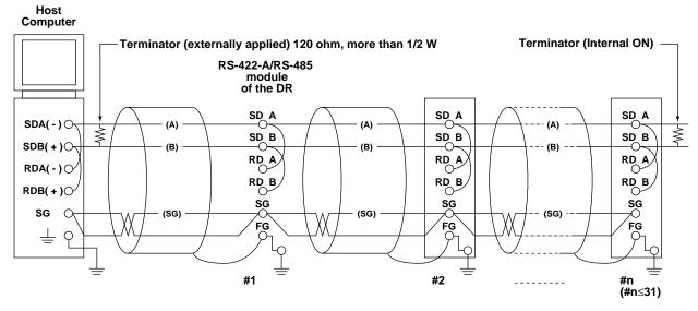
No terminators are inserted between #1 through #n-1 (internal OFF)
