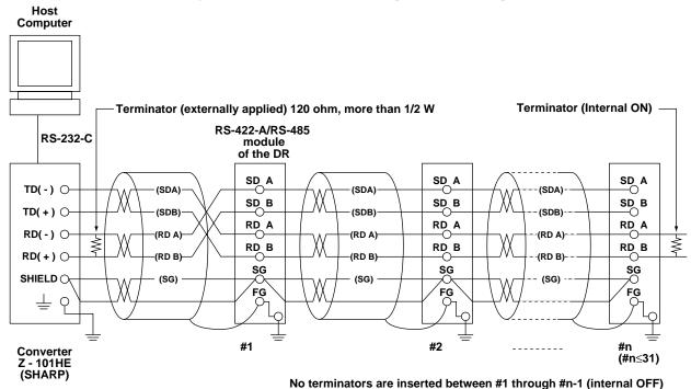
(Diagram below shows the case when the port of the host computer is RS-232-C)
