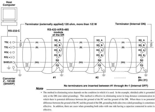
(Diagram below shows the case when the port of the host computer is RS-232-C)
