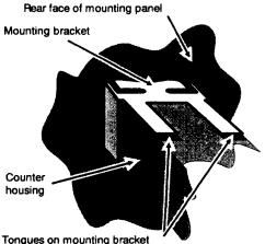
Tongues on mounting bracket engage in ratchet slots on Counter housing
