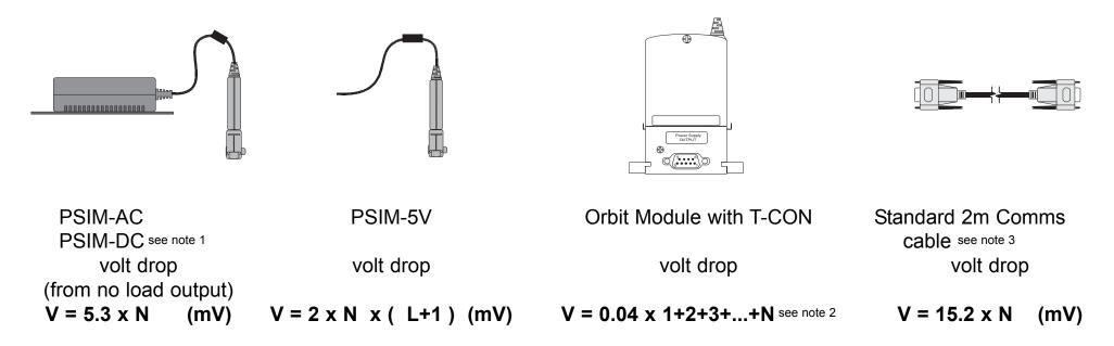
Where N = number of Orbit Modules with T-CON following any particular part above
