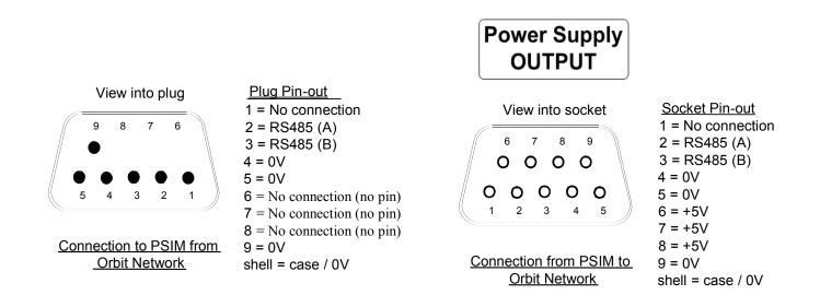
The PSIM will only supply power to the Orbit Modules that follow the PSIM. Some typical configurations are shown. For more information about PSIM and Orbit Network connection, refer to the Applications section.
