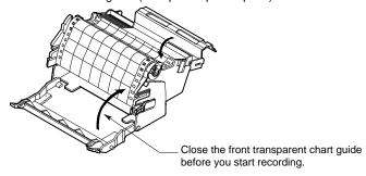
10.Replace the chart cassette back into the recorder case; hang the knurls of the cassette to the grooves of the case, and move the cassette to trap the stopper.
