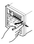
2. Pull and open the display around the hinge.
