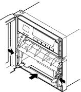
11.Press the **FEED** key on the key panel to assure that the chart moves two or more folds smoothly into the chart receiver. If it moves unsteadily, do the installing procedure again from step (4).
