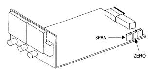
NOTE: Display readings take up to 10 seconds to respond to changes in the zero and span pots.
