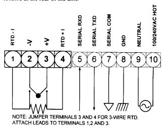
Connect the input power and RS-232 wires to the wire entry locations beneath and perpendicular to the plug-in direction according to figure above.
