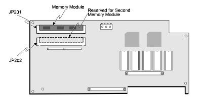
Microprocessor Board (Not all components shown)
