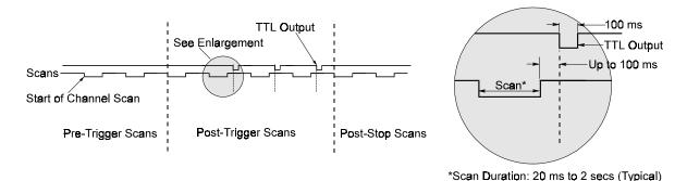
Trigger Timing Diagram
