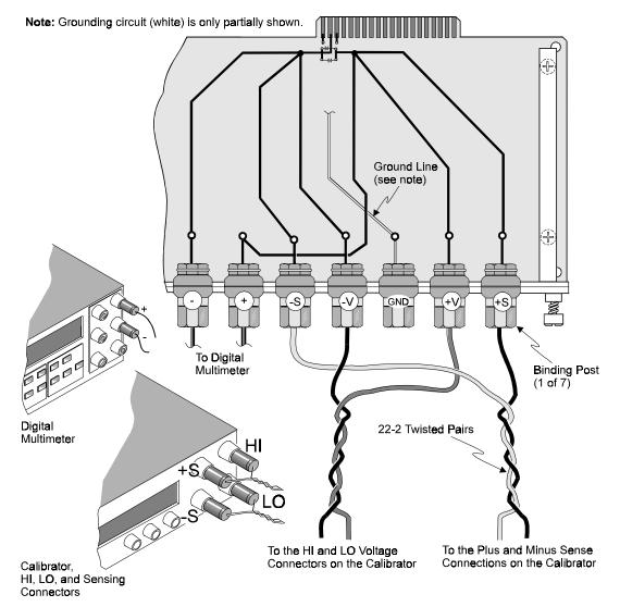
Connections for Main Unit Gain Calibration
