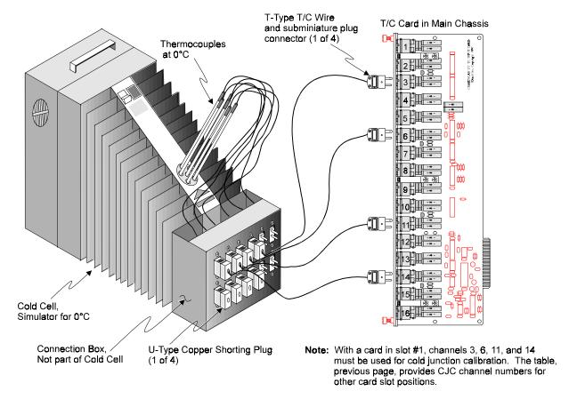
Cold Junction Calibration, Equipment Setup
