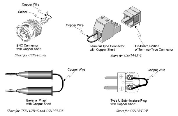
Four Possible Short Types used for Signal Conitioning Card Offset Calibration
