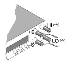
Calibrator, Voltage and Sensing Connections
