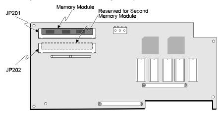
Microprocessor Board (Not all components shown)
