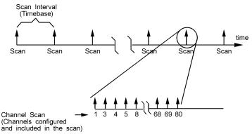
Channel Scan and Scan Interval Definition
