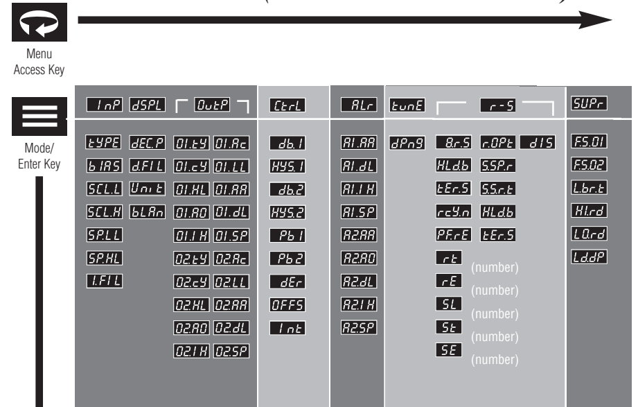
Figure 11. Chart of Series CN8200 Menu System and Security Levels (CONTINUED TO NEXT PAGE)
