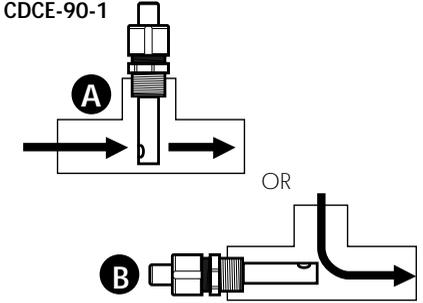
Use caution to avoid air bubble or sediment trapping inside the electrode cavity.
