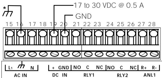
Note: AC/DC power can be connected simultaneously, using DC power as an backup power source.
