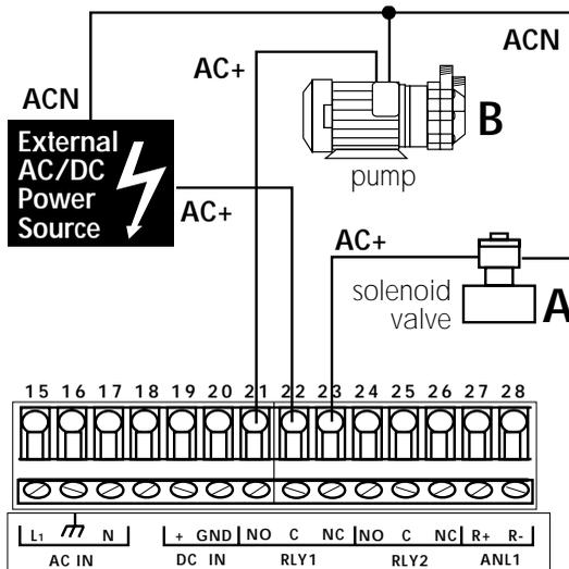
**The Dual Proportional Relay Card** provides a normally open (NO) contact for external device control. The main distinction from the 2-Relay card is the lack of the normally closed (NC) contact.
