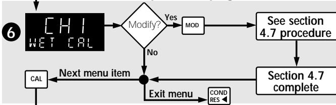
A known solution (sec. 5.6) is required for the "WET CAL" procedure (sec. 4.7).
