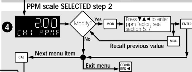
★An internal pure water curve is used for the 10 MΩ to 18 MΩ (0.055 μS to 0.1 μS) range. The factory default setting of 2.00%/°C should be used for this range.
