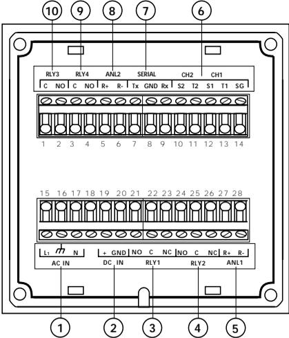
**Note:** Rear terminals accept 18 to 22 AWG wire
