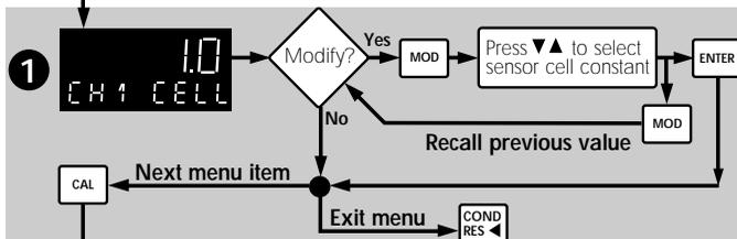
Menu access forces all analog output signals low and temporarily de-energizes available output relays.
