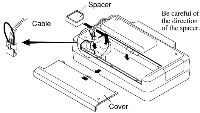
When removing the Ni-Cd battery pack, pull the strap to unplug the connector from the battery housing. Do not pull on the cable of the connector.
