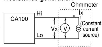
Ix: Current from the constant current source (measured current)
