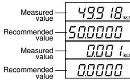
7 Connect a high-accuracy resistance of the specified value and measure the resistance. Correct the value of the calibration point and press [NEXT ENTER] to confirm it.
