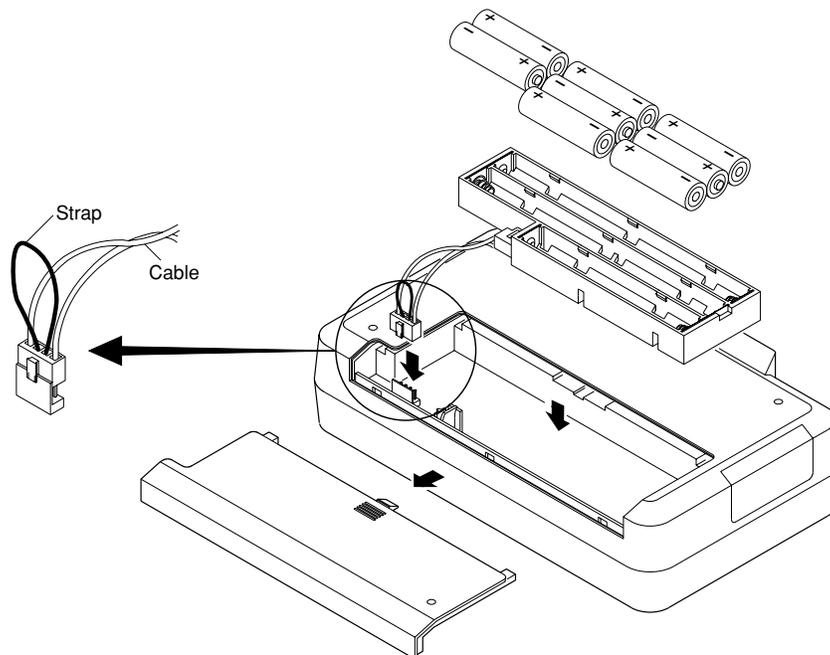
To remove dry cells, pull the strap to unplug the connector from the dry cell storage and remove the dry cell holder. Do not pull on the cable of the connector.
