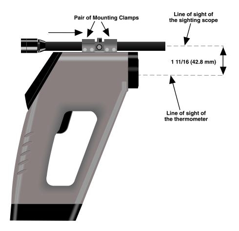
Figure 4-1. Installing the Sighting Scope
