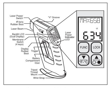
Figure 1-1. OS530/OS520 Series Handheld Infrared Thermometer Front View
