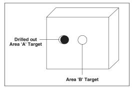
Figure C-2. Determining Emissivity with a Drilled Hole
