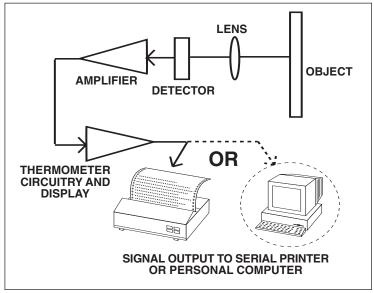
Figure A-1. Infrared Thermometer Block Diagram
