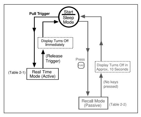
Figure 2-12. General Operational Block Diagram
