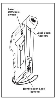
Figure 3-1. Rear View of the Thermometer
