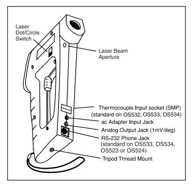
Figure 1-3. OS530 Series Handheld Infrared Thermometer Rear View
