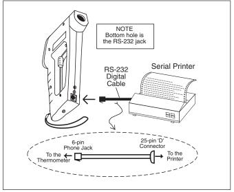
Figure 2-14. Serial Printer Hookup
