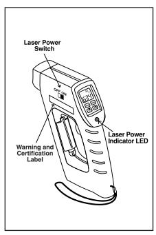
Figure 3-2. Front View of the Thermometer
