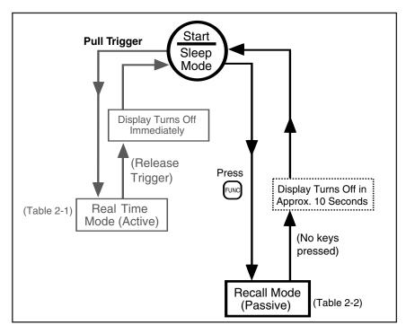
Figure 2-16. General Operational Block Diagram
