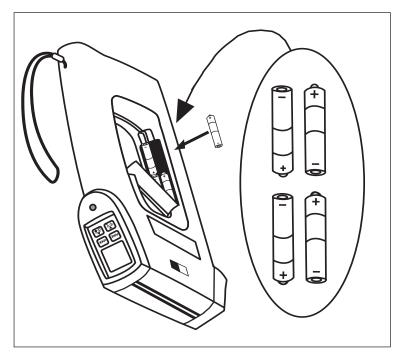
Figure 2-1. Installing the Batteries
