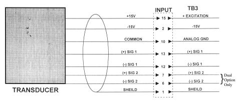
USING INTERNAL ±15VDC SUPPLY
