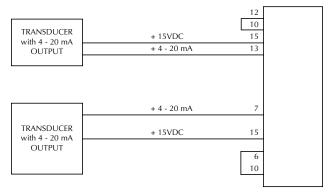
Note: (+) (-) signal input level is selectable by switch(s) on rear of unit. Input range 0 to + 20mVDC, + 5VDC, + 10VDC, and 4-20 mA.
