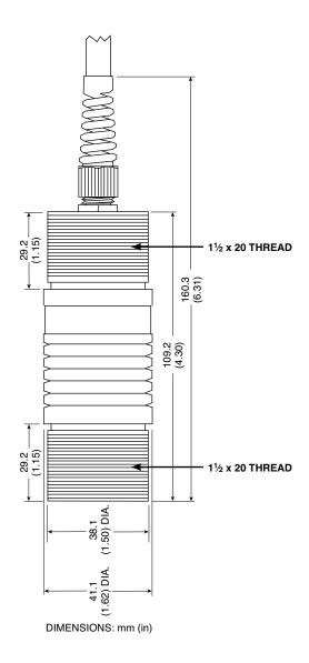
Fig. 2-1. Sensor Head Dimensions
