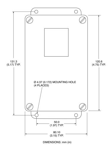
Fig. 2-2. Plastic Housing Dimensions
