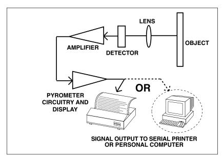
Figure A-1. Infrared Thermometer Block Diagram
