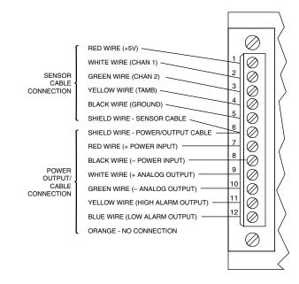
Figure 3-2. OS550A-BB Wire Connection
