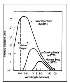
Relative emission from a blackbody versus wavelength. The area under the curve corresponds to the total energy, and is proportional to the absolute temperature to the 4th power. The peak of the spectral distribution curve shifts to shorter wavelengths as the temperature increases. <u>Wien's Displacement Law</u> describes the exact mathematical relationship between the temperature of a blackbody and the wavelength of the maximum intensity radiation.
