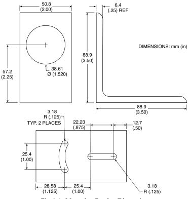
Fig. 2-4. Mounting Bracket Dimensions
