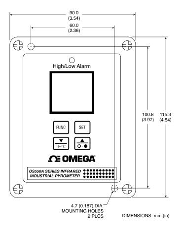
Fig. 2-2A. Aluminum Housing Dimensions
