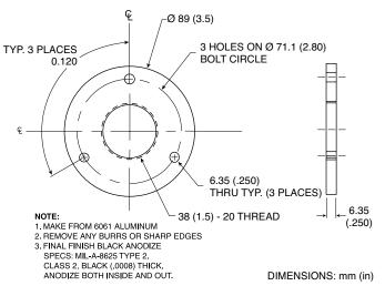
Fig. 2-6 Mounting Flange Dimensions
