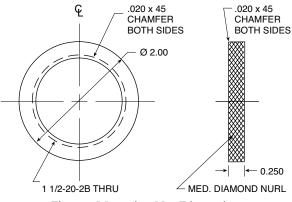
Fig. 2-5 Mounting Nut Dimensions
