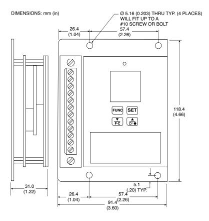
Fig. 2-3. OEM Style Main Display with Mounting Plate
