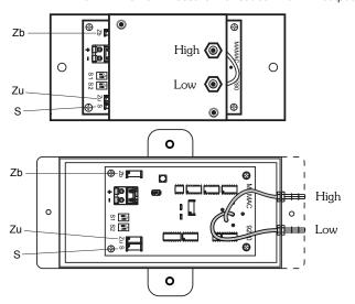
PX274/275/277/278 pressure transducers with 4-20 mA output are powered with a12-40 VDC supply.
