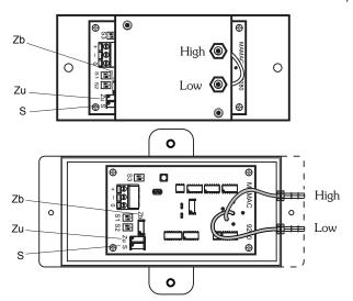
PX274/275/277/278 pressure transducers with VDC output are field selectable 0-5 VDC or 0-10 VDC output and can be powered with either a 12-40 VDC or 12-35 VAC
