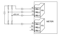
Figure 7-17. Bridge Input With External Sensor Excitation
