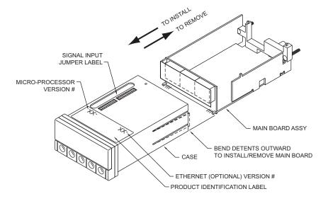
Figure 5-2. Board Assembly Removing/Installing Detail
