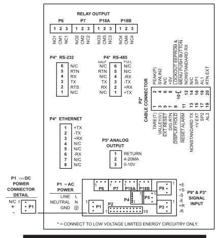
Figure 4-2. Connector Label (AC-Powered and DC-Powered Detail)
