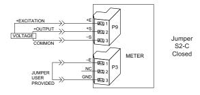
Figure 7-15. 3-Wire Voltage Input With Sensor Excitation
