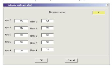
This scaling method based on 2 Input values entered with 2 corresponding readings. Up to 10 Linearization Points can be selected to customize the transducer curve.
