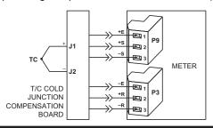
Figure 7-8. Directly-Connected Thermocouple
