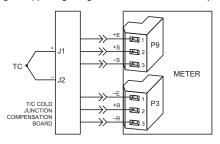
Figure 7-21. Directly-Connected Thermocouple
