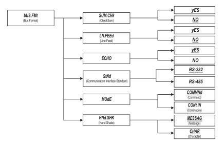
Bus Format determines Communication Standards and Command/Data Formats for transferring information into and out of the controller via the Serial Communication Bus. Bus Format submenus essentially determine how and when data can be accessed via the Serial Communications of the device.
