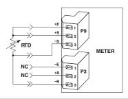
Figure 7-11. RTD Connections with 4-wire RTD
