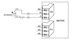
Figure 7-12. Current Input Without Sensor Excitation
