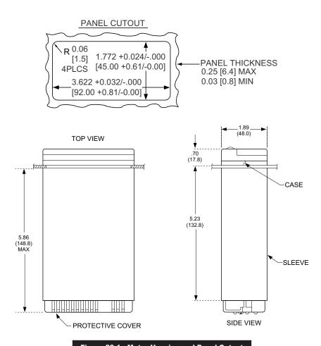
Figure 33-1. Meter Housing and Panel Cutout
