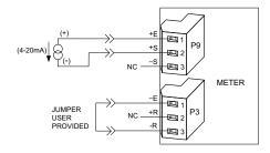
Figure 7-2. Current Input With Sensor Excitation
