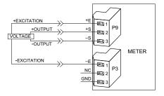
Figure 7-16. 4-Wire Voltage/Bridge Input With Sensor Excitation
