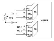
Figure 7-9. RTD Connections with 2-wire RTD
