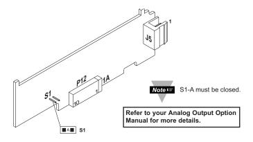
Figure 5-9. Analog Output Option Board
