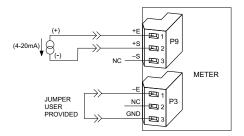
Figure 7-13. Current Input With Sensor Excitation
