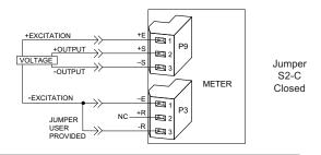
Figure 7-5. 4-Wire Voltage Input With Sensor Excitation
