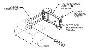
Figure 7-20. Installation of Thermocouple Cold-Junction Compensation Board Assembly
