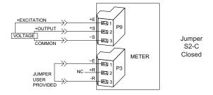
Figure 7-4. 3-Wire Voltage Input With Sensor Excitation
