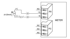
Figure 7-1. Current Input Without Sensor Excitation
