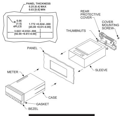
Figure 5-10. Panel Mounting Assembly
