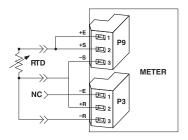
Figure 7-10. RTD Connections with 3-wire RTD
