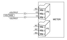
Figure 7-3. Voltage Input Without Sensor Excitation
