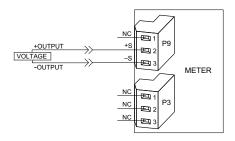
Figure 7-14. Voltage Input Without Sensor Excitation
