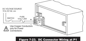
For DC low voltage power option, in order to maintain the same degree of protection as the standard AC high voltage input power units, always use a Safety Agency Approved DC power source with the Overvoltage Category and polution degree.
