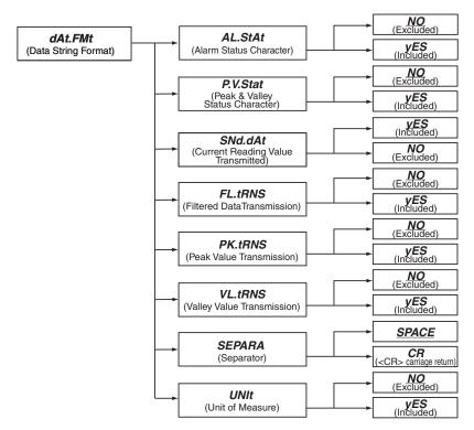
With this "dAt.FMt" Data Format Configuration Submenu, user can select and setup all the parameters to be transmitted via the optional (RS-232 /RS-485) Serial Communication Board.
