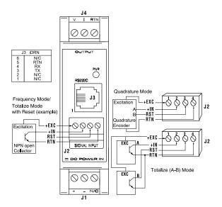
**Note:** When connecting a pulse signal, ensure that the input signal voltage is less than or equal to the rating. The unit may be damaged if the input voltage exceeds the maximum rating.
