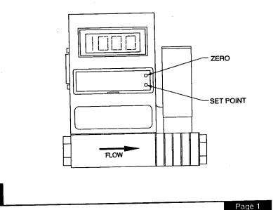
The versatile FMA-1900 product digitally displays the mass flow rate directly in engineering units or percent of full scale.
