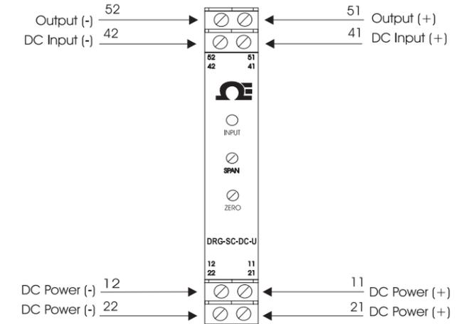
Figure 3: Wiring diagram for both DRG-SC-DC-U.
