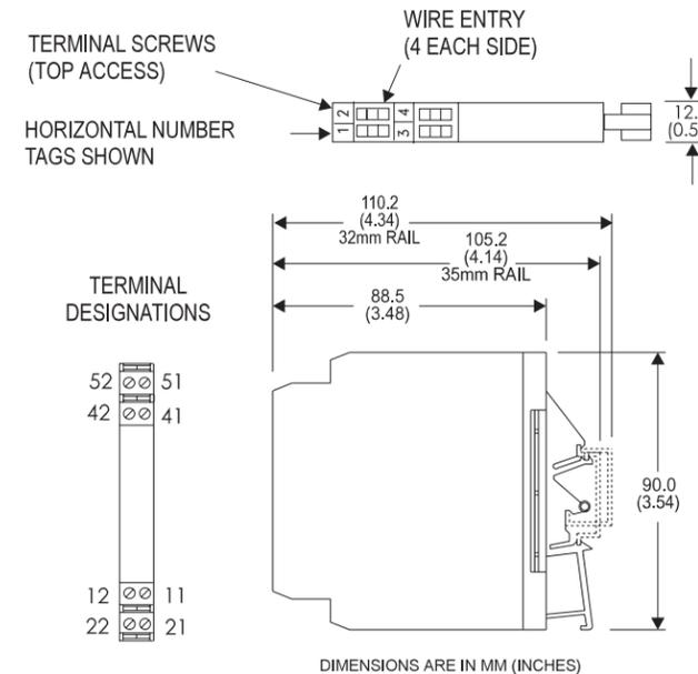
**Figure 4: Mechanical dimensions for both DRG-SC-DC-U and DRG-SC-DC-B.**
