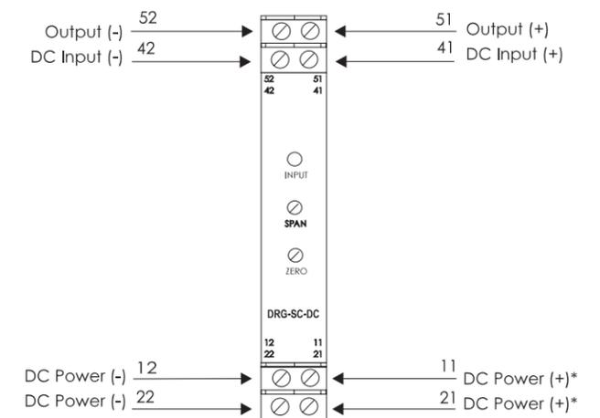
**Figure 5: Wiring diagram for both DRG-SC-DC-U and DRG-SC-DC-B**
