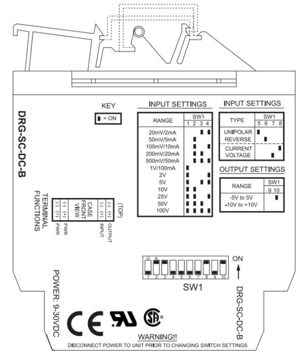
**Figure 3: DRG-SC-DC-B factory calibration; 4-20mA, unipolar input, normal operation, -10 to +10V output.**
