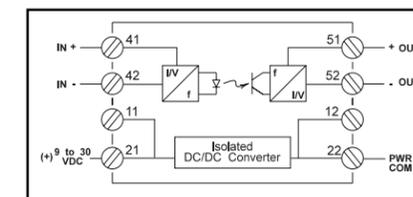
Figure 1: DRG-SC-DC block diagram.
