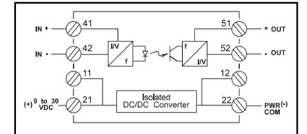
Figure 1: DRG-SC-DC-U block diagram.
