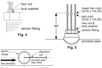
The flow sensor alignment rod MUST be parallel to the process pipe as shown. Fig. 6
