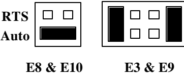
Figure 8 - RS-485 'Auto' Enabled, with 'Echo'
