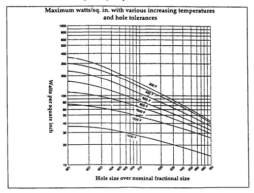
The watt densities are based on a unit installed in mild steel. Different materials affect the above values, i.e. the lower the thermal conductivity of the material, the lower the maximum allowable watts per square inch.
