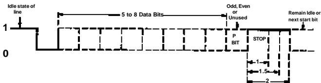
Figure 9 - Asynchronous Communications Bit Diagram
