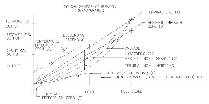
Terminal Non-Linearity (N/L): computed from deviations of ascending theoretical data from a straight line connecting the zero and full scale points.
