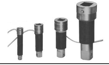
The OMEGA® TQ103 Series socket extension torque sensor is ideal for installation between a socket and drive to measure or verify bolt torque. The sensor can measure torque in both clockwise and counterclockwise directions. Any electronic display or control device which is compatible with strain gage transducers may be used with the sensor. The sensors are available in 1/4", 3/8", 1/2", and 3/4" square drives.
