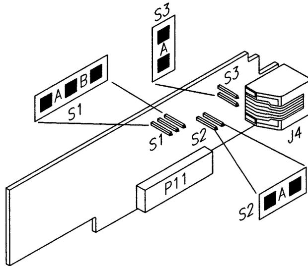
Figure 15-2. RS-485 Serial Communications Board
