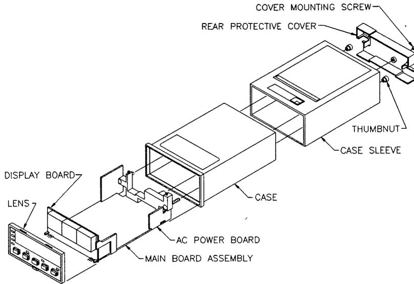
**Figure 2-2. Exploded View of Meter with Optional Housing**
