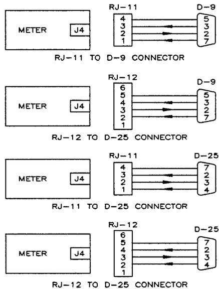
Figure 15-3. 4-Wire RS-232 Connections
