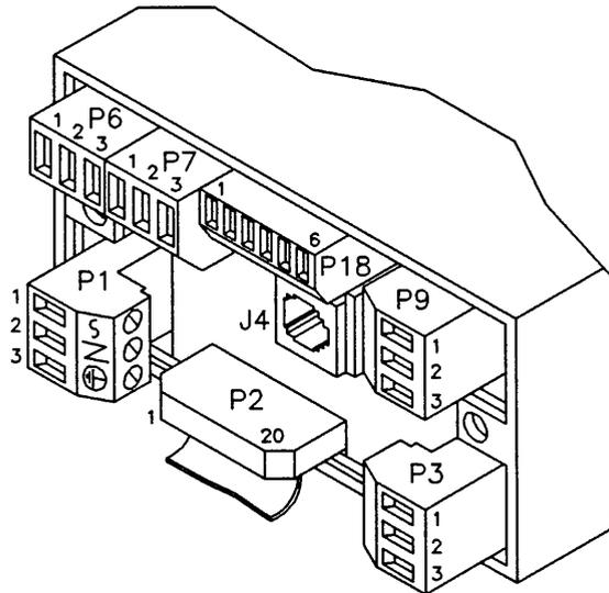
**Figure 7-1. Rear View of Meter with 4-Relay Board and Serial Communications**
