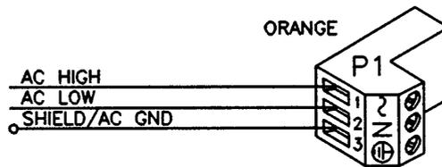
Figure 3.2 AC power plug wiring
