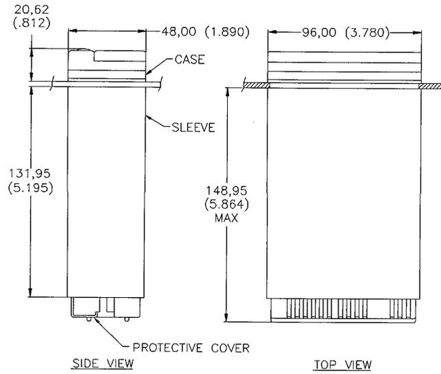
**Figure 21-3. Meter Dimensions with Standard Bezel**
