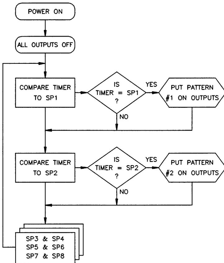
Figure 14-7. INDPAT Mode Flowchart
