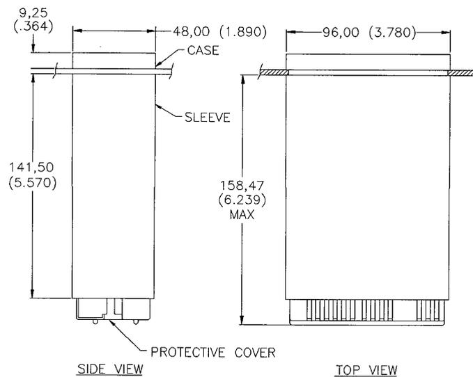
**Figure 21-5. Meter Dimensions with Optional Housing**
