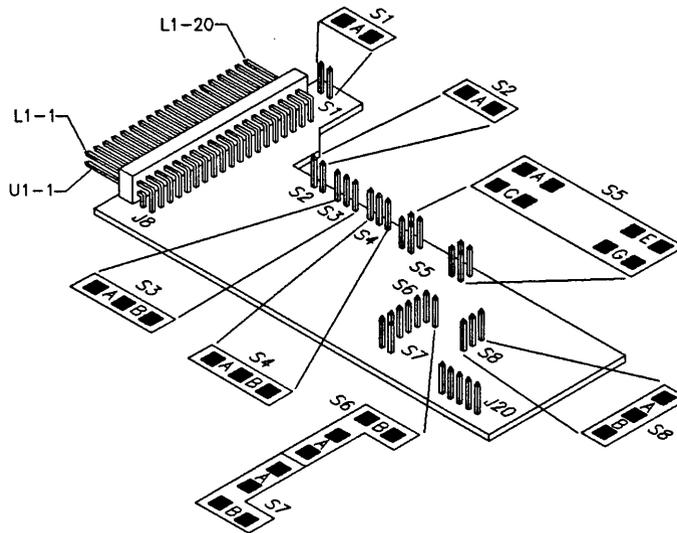
**Figure 16-1. BCD Board Jumper Locations**
