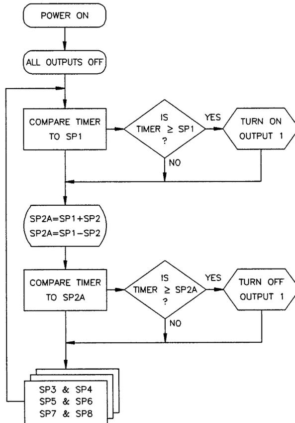
Figure 14-3. ELAPSE Mode Flowchart
