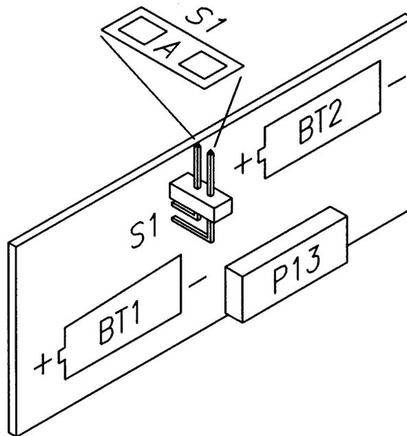
Figure 19-1. Battery Board Jumper and Battery Location
