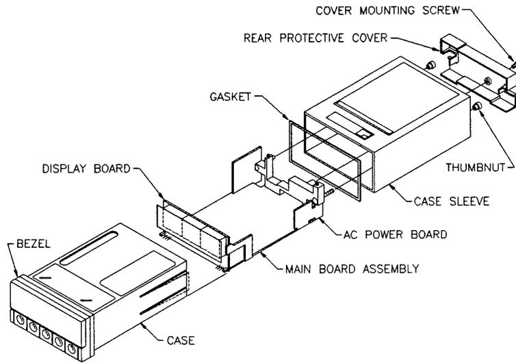
**Figure 2-1. Exploded View of Meter with Standard Bezel**
