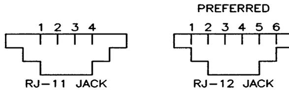
Figure 15-4. RJ-11 and RJ-12 Connectors
