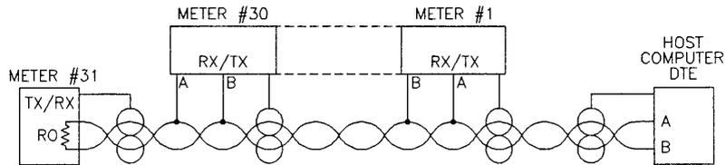
Figure 15-5. Multi-Point Half-Duplex RS-485 Connection
