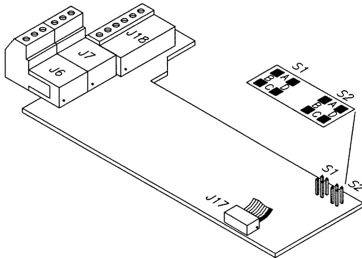
Figure 18-1. 4-Relay Board Jumper Locations
