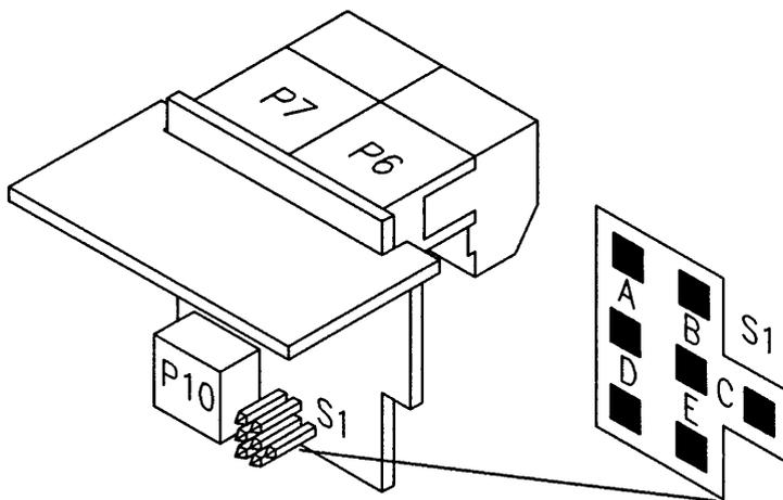
Figure 17-1. Dual Relay Output Board
