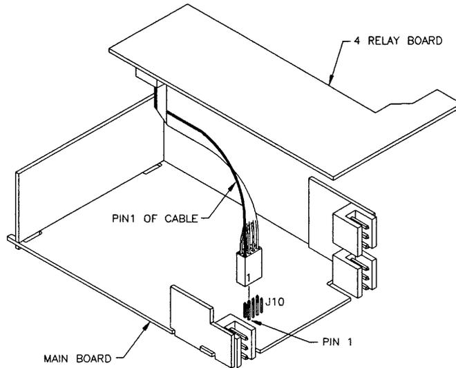
Figure 18-2. 4-Relay Board Installation
