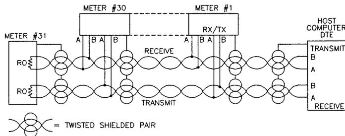
**Figure 15-6. Multi-Point Full-Duplex RS-485 Connection**
