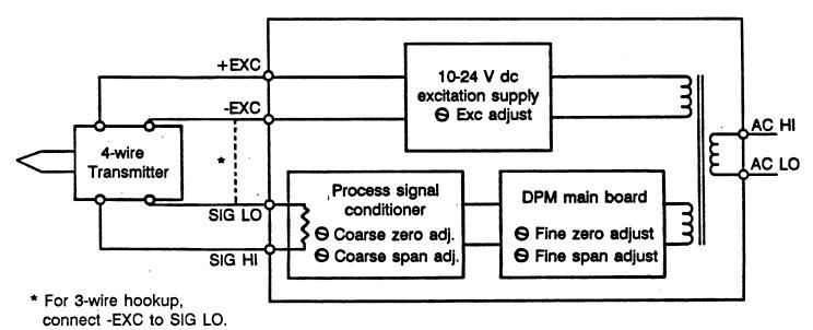
Figure 9-2 Four-wire Connection
