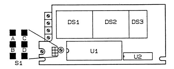
Figure 5-1 Display Board Jumper Locations
