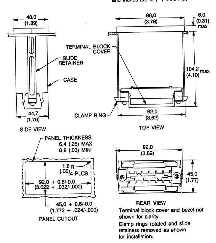
Figure 3-1 DIN Case Dimensions
