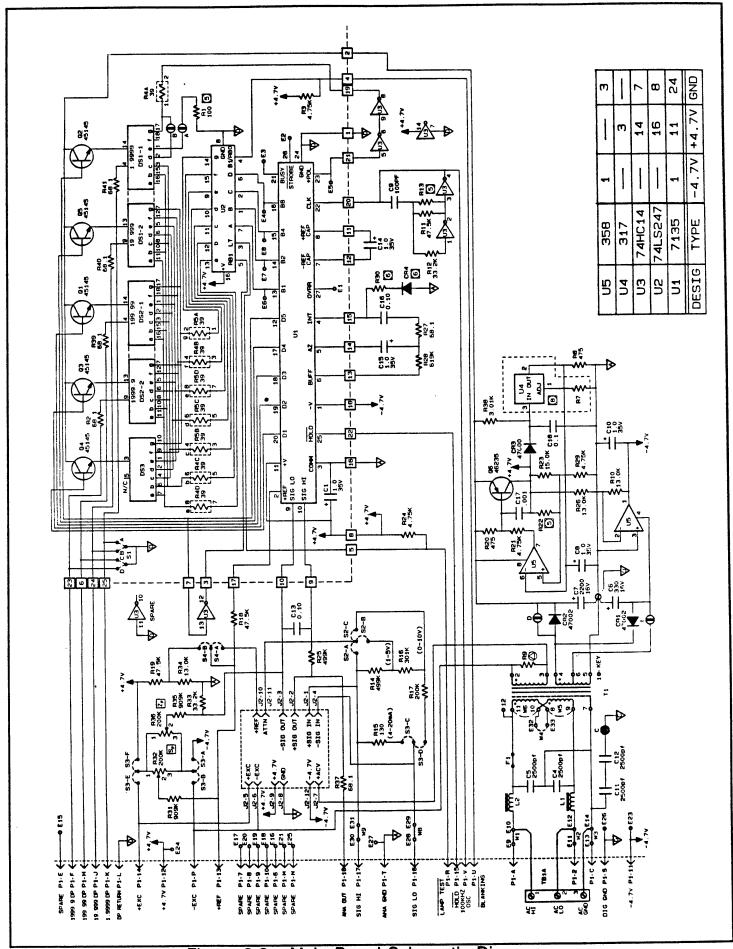
Figure 8-2 Main Board Schematic Diagram
