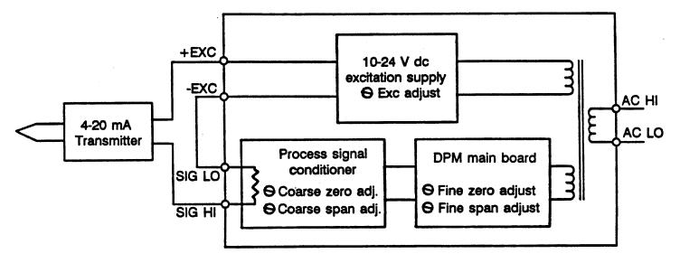
Figure 9-1 Two-wire Connection
