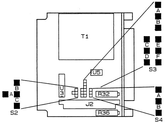
Figure 5-2 Main Board Jumper Locations
