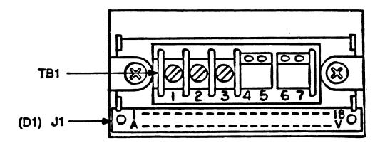
Figure 4-2 Rear View of Case with Connectors
