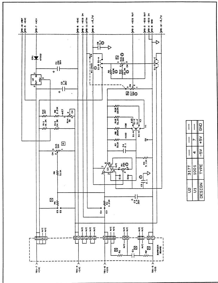
Figure 8-6 Plug-in Card Schematic -S Diagram
