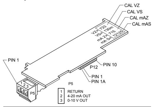
Figure 12-1. Analog Option Board and Connection Diagram at P5
