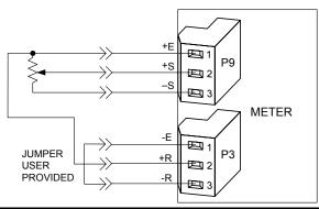
Figure 7-6. Potentiometer Connections with Internal Power Supply and Ratio Measurement.
