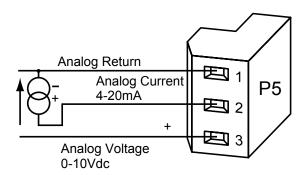
Figure 12-2. Isolated Analog Output Board Wiring Connections.
