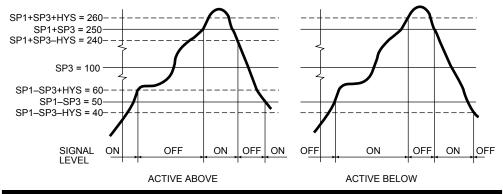
Figure 10-6. Band Deviation for both Active Above and Active Below
