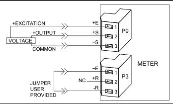
Figure 7-4. 3-Wire Voltage Input With Sensor Excitation
