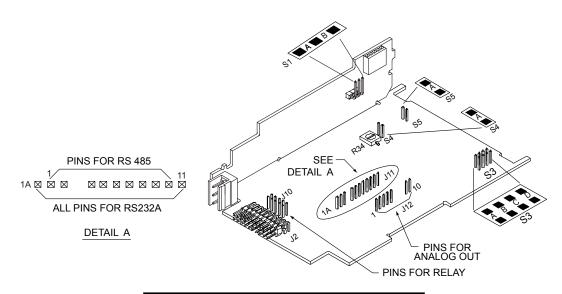
Figure 5-7. dc-Powered Main Board
