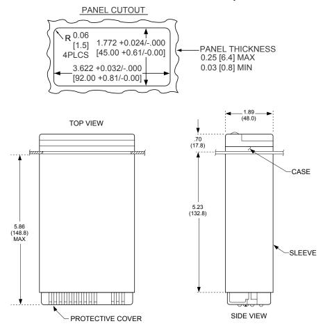
Figure 17-1. Meter Housing and Panel Cutout.
