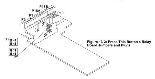
The table below shows which jumpers are assigned to each relay. Defaults have asterisks. re 4 Relay Output Board Wiring Connections.
