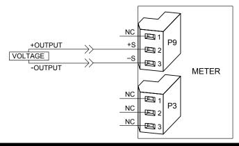
Figure 7-3. Voltage Input Without Sensor Excitation
