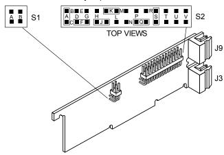
Figure 6-1. S1 and S2 Jumper Locations on Signal Input Board
