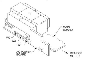
Figure 5-3. Transformer Jumpers
