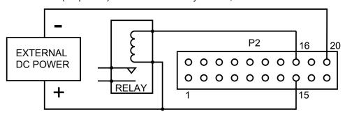
Figure 15-2. Connection of External Power for Setpoint Transistors
