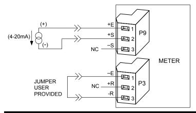
Figure 7-2. Current Input With Sensor Excitation
