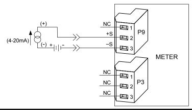
Figure 7-1. Current Input Without Sensor Excitation
