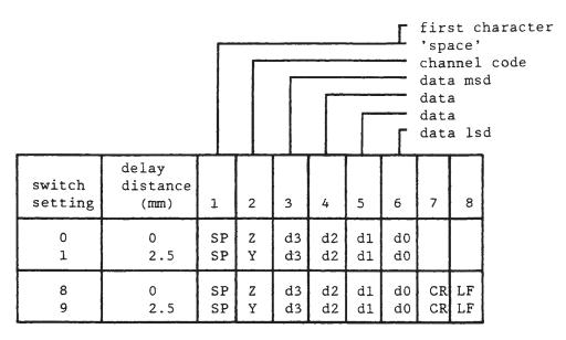
Figure 5-2. Switch setting and data format
