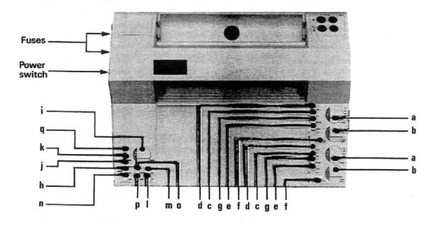
Figure 3-1. Location of Operator Panel Functions
