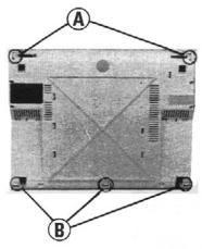
A: Ridges to be opened by screwdriver. B: Ridges to be opened by hand.
