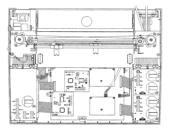
Figure 5-1. Mainboard Layout
