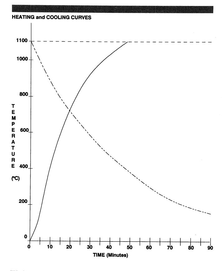
TEST CONDITIONS: Nominal Line Voltage; No Load In Muffle; Full Power Applied To Muffle for heating. No power applied to muffle for cooling.
