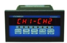
Once the correct pass-code has been entered, the display shows 'SYS CH', with 'CH' blinking. At this point the operator may choose between making channel settings (CH), or system settings (SYS). Use 'v key to toggle between CH and SYS modes. When the desired mode is blinking, press SETUP key to begin setup of parameters for that mode. 'SYS' Parameter List
