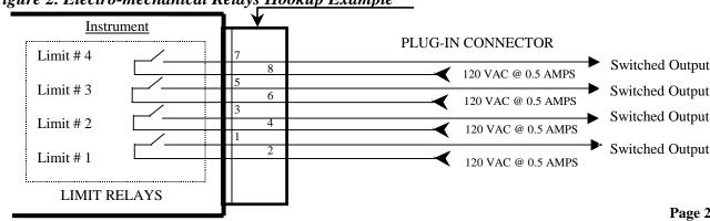
Figure 2. Electro-mechanical Relays Hookup Example
