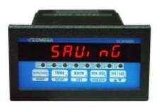
permanent storage. It is important that the above step be performed any time changes are made to the configuration of the unit and before power is removed. If not done so, all the new changes will be lost. The unit will, however, maintain the old settings.
