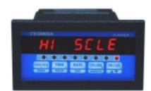
key and then pushing it again will decrement the value ( $^v$  key works as a toggle -- alternating between increment and decrement). To change the next digit first push the <NEXT> key. This will advance the flashing to the following digit. Use  $^v$  key to change the value. After the desired High Scale setting is displayed, push **SETUP** key to enter that setting and go to setup Low Scale.
