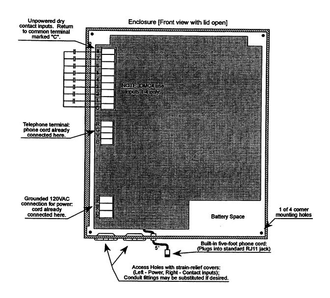
Figure 2-2. Electrical Connections for Models OMA-C16, OMA-C24 & OMA-C32
