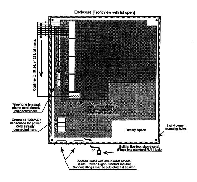
Figure 2-1. Electrical Connections for Models OMA-C4 & OMA-C8
