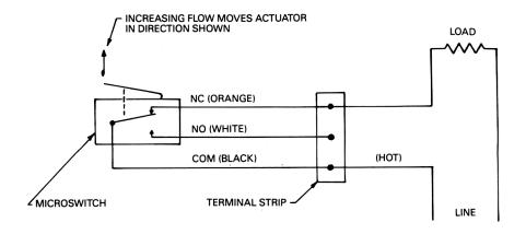
Figure 2: Wiring Schematic for power applied to load when flow is LESS than set point (power to load interrupted when flow is GREATER than set point).
