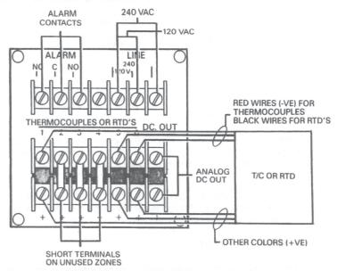
Figure 2-2. Wiring Diagram
