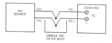
Figure 4-2. Thermocouple Calibration
