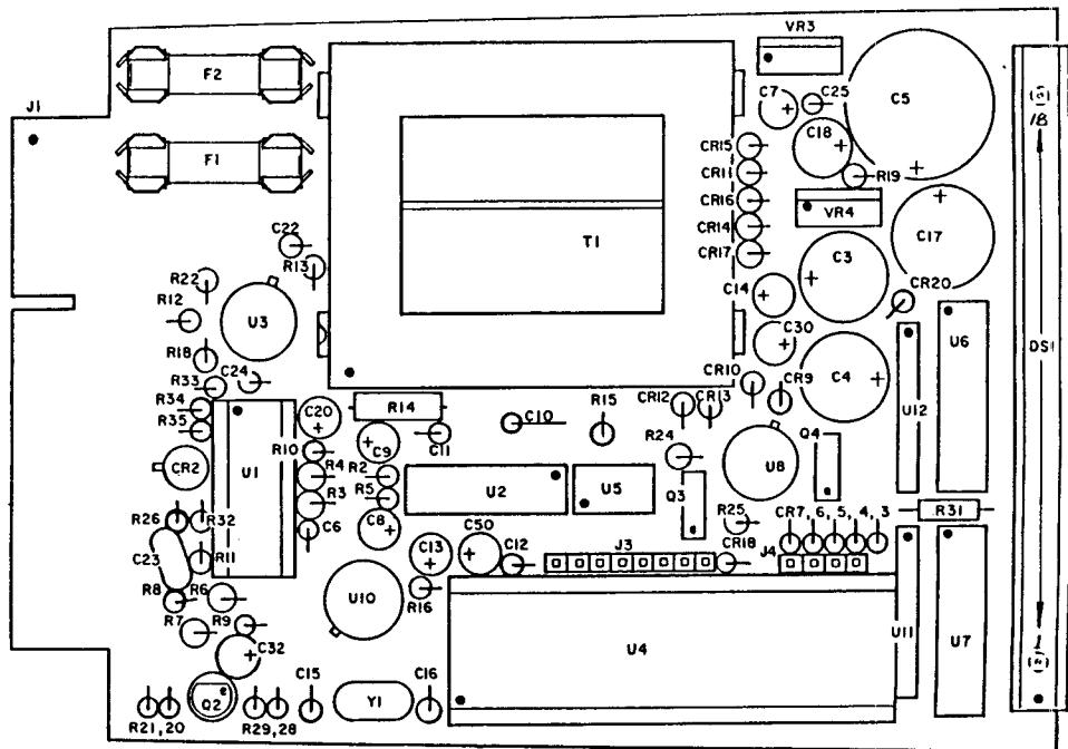
Figure 9. Main P.C. Board Assembly
