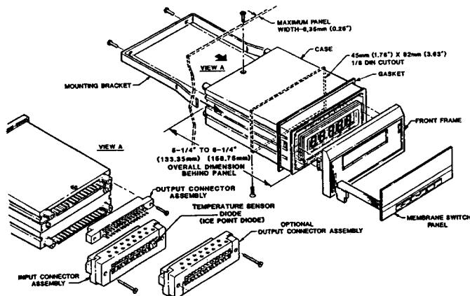
Figure 1. Unit Installation and Assembly
