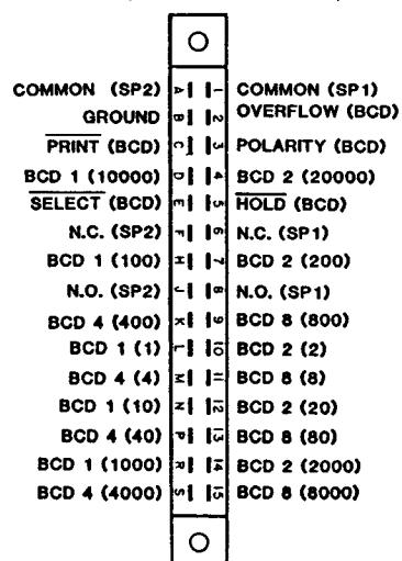
Figure 4B. P2 Edge Connector Option R (Relays Output) and Option B (BCD Output)
