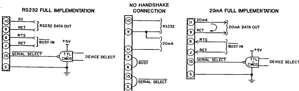
Figure 6. Various Option S Connections
