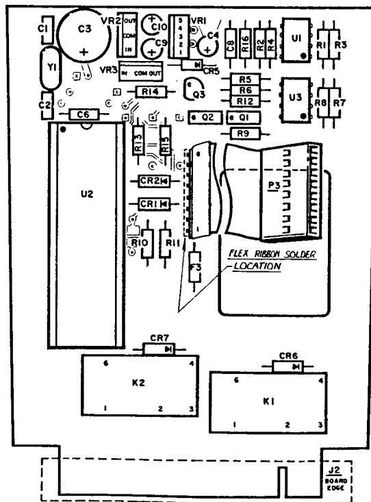
**Figure 11. RB Option Board Assembly**
