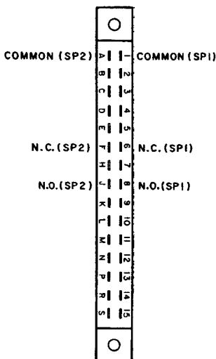
Figure 4A. P2 Edge Connector Option R (Relays Output)
