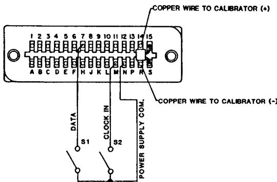
Figure 3. Recalibration Connections (P1 Connector)
