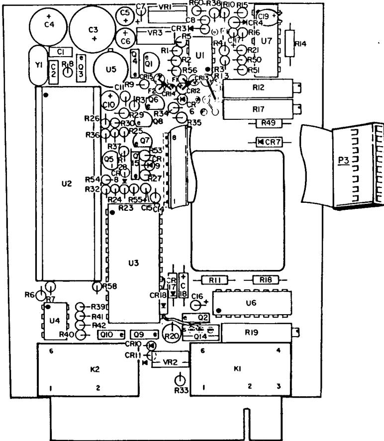
Figure 13. RS, RA, RSA Option Board Assembly
